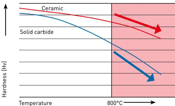
Cemented carbide end mills are significantly reduced in strength when exceeding 800°C. However, the strength of ceramic end mills is not affected and therefore can be used at the high speeds and depths of cut required to generate sufficient heat to enable effective machining.
