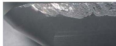
Example of thermal cracking
