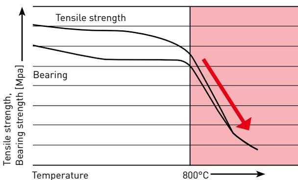
Ni based difficult-to-cut heat resistant alloys such as Inconel 718 soften at temperatures exceeding 800°C. At these temperatures, difficult-to-cut materials become easier to machine because their bearing and tensile strengths are lowered. Ceramic end mills can work effectively at these high temperatures and self generate the heat required to soften the material to be machined by using ultra-high feeds and speeds.
